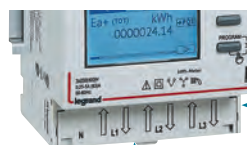
Clear marking indicating the terminal position and wiring direction.
