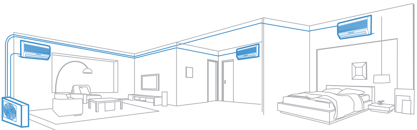
MULTI AIR CONDITIONING UNIT SYSTEM
